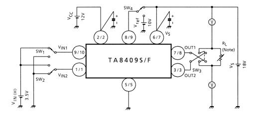
Note: Calibrate I<sub>OUT</sub> to 0.2 / 0.4 A by R<sub>L</sub>.
