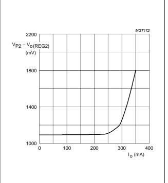
Fig.7 Dropout voltage of V<sub>P2</sub> as a function of the output current of regulator 2.
