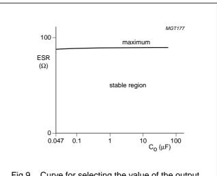
Fig.9 Curve for selecting the value of the output capacitor for regulators 1, 3, 4 and 5.
