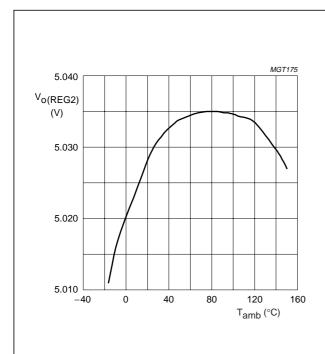
Fig.4 Output voltage of regulator 2 as a function of the ambient temperature.
