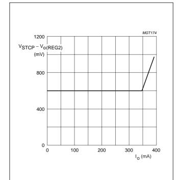
Fig.6 Dropout voltage of V<sub>STCP</sub> as a function of the output current of regulator 2.
