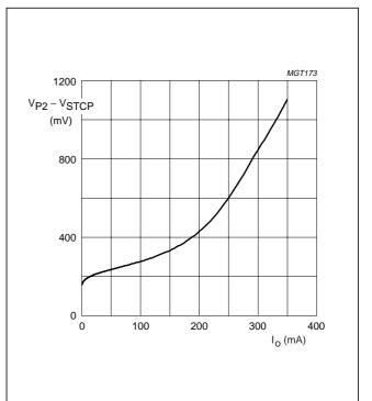
Fig.5 Voltage drop of  $V_{P2}$  as a function of the output current of regulator 2.
