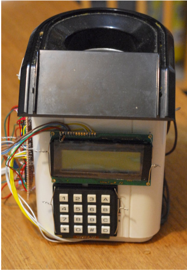
Terran's Pi controlled coffee roaster ( http://adafru.it/aLm )
