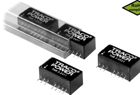
The TMR-3 series is a new family of isolated 3W dc-dc converter modules with regulated output, featuring wide 2:1 input voltage ranges. The product comes in a ultra-compact SIP-8 plastic package with a small footprint occupying only 2.0 cm<sup>2</sup> (0.3 square in.) of board space.
