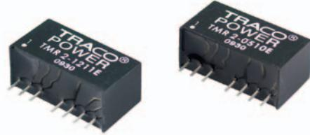
The TMR-2E series is a family of isolated 2 W dc-dc converter modules with regulated output, featuring wide 2:1 input voltage ranges. The product comes in a compact SIP-8 plastic package with small footprint occupying only 2.0 cm<sup>2</sup> (0.3 square in.) of board space.
