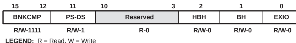
Figure 6. Bank-Switching Control Register (BSCR), MMR Address 0029h
