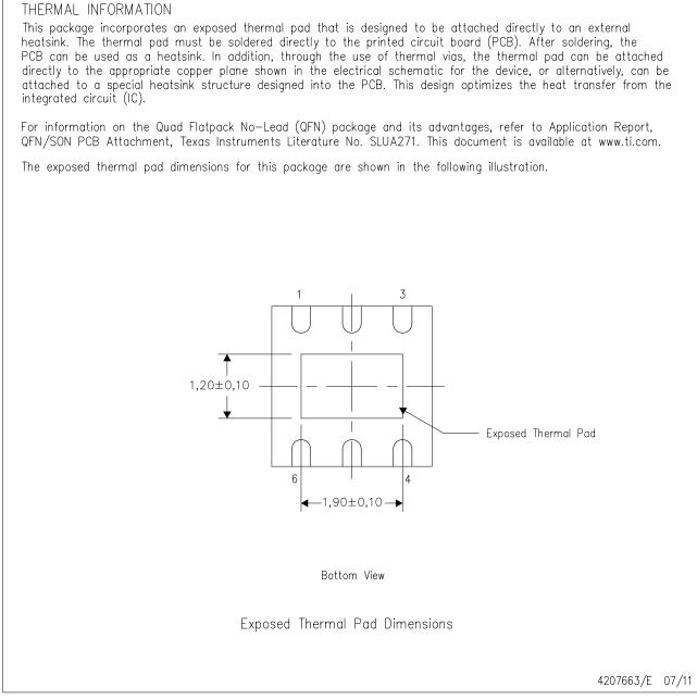
NOTE: All linear dimensions are in millimeters
