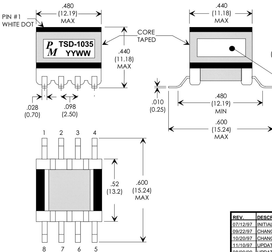
**FIGURE 3: RECOMMENDED PCB LAYOUT DIMENSIONS IN INCHES (mm)**
