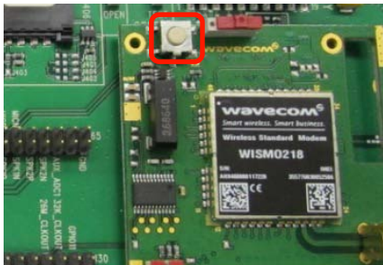
Figure 47. AirPrime WISMO2x8 Embedded Module ON/~OFF Switch on the WISMO2x8 Socket Board
