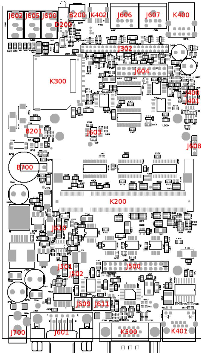
The diagram above shows connectors, jumpers and other interfaces layout of Voipac PXA270 baseboard. Voipac PXA270 baseboard is 4 layers pcb design with parts on top side only. The PCMCIA and CF sockets are on bottom side.
