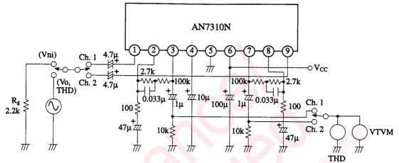
Note 1) THD is measured by equipment with 400Hz low pass filter Note 2)  $V_{ni}$  is measured by equipment with 15Hz ~ 30kHz band pass filter
