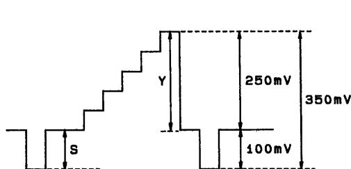
$$LS = \frac{S \text{ [mV]}}{Y \text{ [mV]}} \times 100 \text{ [%]}$$
