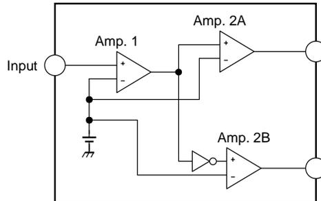
**Figure 1 Block Diagram**
