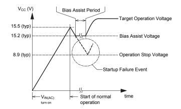
Figure 4. VCC during startup period
