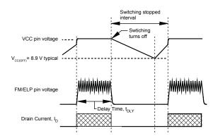
Figure 17. Waveforms during OLP operation
