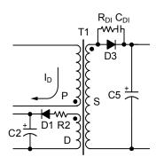
Figure 25. Damper resistor example
