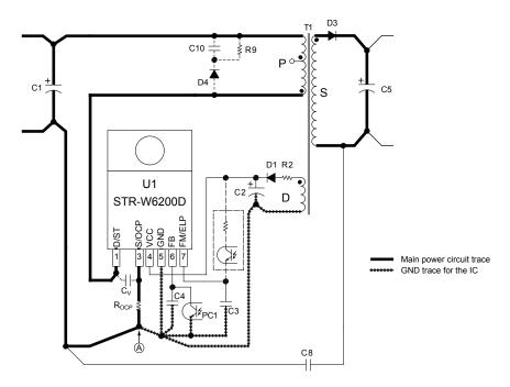
Figure 27. Peripheral circuit example around the IC
