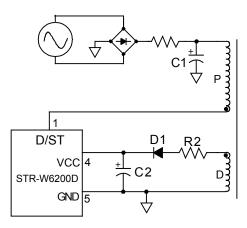
Figure 2. VCC pin peripheral circuit
