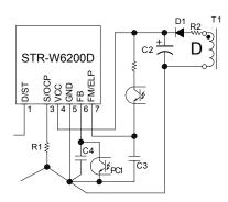
Figure 22. FB pin peripheral circuit
