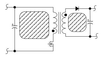
Figure 26. High-frequency current loops (hatched areas)
