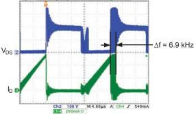
Figure 9. V<sub>DS</sub> and I<sub>D</sub> waveforms in frequency modulation
