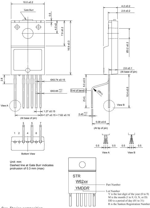
Pin treatment Pb-free. Device composition compliant with the RoHS directive.
