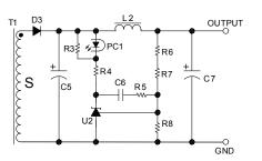
Figure 21. Peripheral circuit around secondary shunt regulator (U2)
