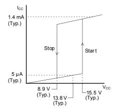
Figure 3. VCC versus ICC
