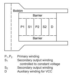
Figure 7. Winding structural example (a)
