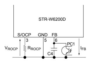
Figure 12. FB pin peripheral circuit
