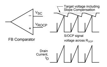
Figure 13. Drain current,  $I_{\text{D}},$  and FB comparator operation in steady operation
