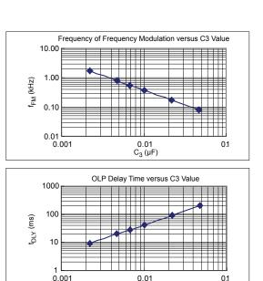
Figure 23. The relationship between t<sub>FM</sub>, t<sub>DLY</sub>, and C3 (calculated values)
