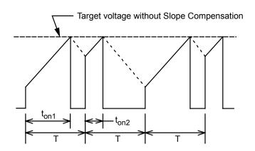
Figure 14. Drain current,  $I_D$ , waveform in subharmonic oscillation
