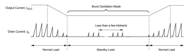
Figure 11. Automatic-Standby mode operation
