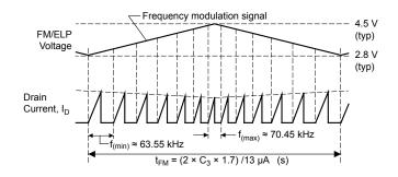
Figure 10. FM/ELP pin voltage and frequency modulation period
