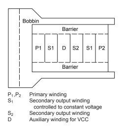
Figure 8. Winding structural example (b)
