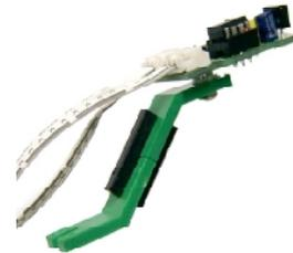
A12.2 Loosen a screw that attach the RBX-877 board with Right angle joiner and insert ZX-08 structure from step A12.1 to space between screw and RBX-877 board. Tighten this screw again for locking the structure. Make same method with another ZX-08 structure.
