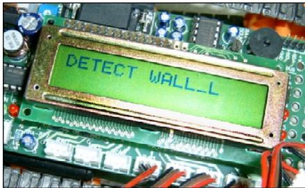
**Figure A13-1** Shows testing of ZX-08 on LCD of Robo-PICA
