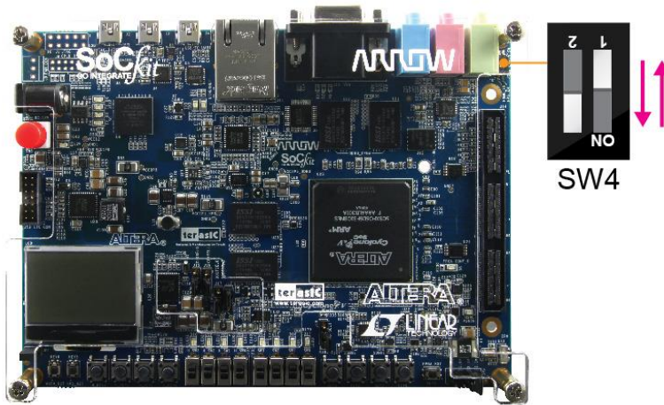
Figure 3-2 JTAG Chain and Setup Switches
