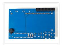
Flip over the assembly, carefully. Then solder in the 16 or 18 pins of header
