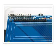
Finally, we place the LCD. Break off a piece of 18 or 16 pin header from the stick in the kit. If you have an RGB display, you'll need 18, for a blue&white you'll need 16
