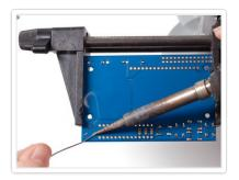
Flip over the PCB and solder in the three legs of the potentiometer
