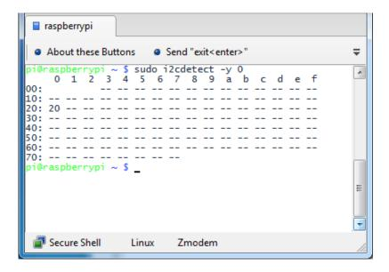
This will search /dev/i2c-0 or /dev/i2c-1 for all address, and if an Adafruit LCD Plate is connected, it should show up at **0x20**
