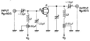
L1:1mmø tin-plated wire, air core 10mmø 4.5T L2:1mmø tin-plated wire, air core 10mmø 3.5T
