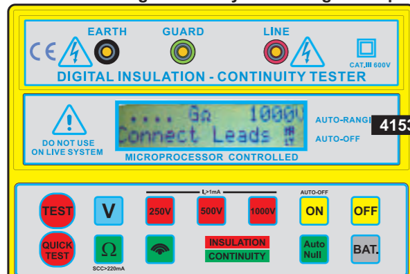
4153IN interactive display asking to connect leads.
