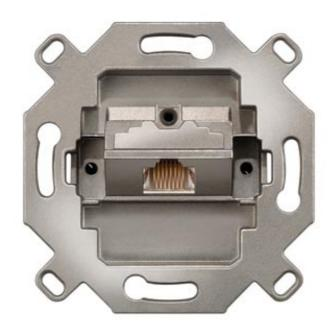
UAE OUTLET BOX CAT.5E, 1X8-POLE W. INCLINED OUTLET RJ45 W. LSA PLUS CONNECTION METHOD FOR SCREW FIXING SHIELDED, F.DELTA PROGRAMS
