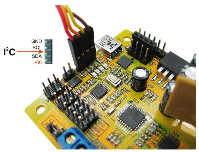
Connect the +V, SCL, SDA and Gnd of the external logic to the +VI, SCL, SDA and GND pins of the T'REX I<sup>2</sup>C interface. The T'REX will automatically translate the voltage. The interface includes 10K pullup resistors although external pullup resistors can be added if required.
