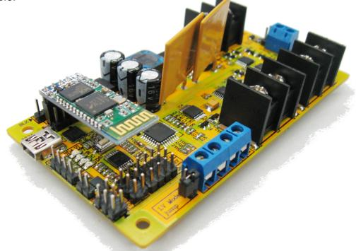
If the bluetooth module is detected the sample code will automatically set the baud rate to 9600, the name to "T'REX" and the pin number to "1234".
