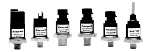
Model MLH pressure sensors combine the latest in Application Specific Integrated Circuit (ASIC) technology with proven media isolated metal diaphragm design. This digitally compensated sensor offers an unparalleled value and performance combination making it the ideal pressure sensing solution for demanding applications. Fully temperature compensated, calibrated, and amplified, the MLH is available in 50 psi to 8,000 psi pressure ranges.
