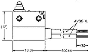
**Note:** UL1007 AWG24 wires are used for UL/CSA approved models.
