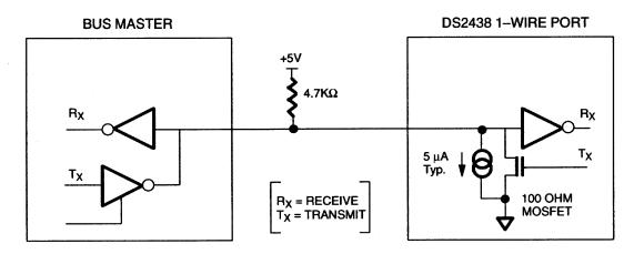
The idle state for the 1 wire bus is high. If for any reason a transaction needs to be suspended, the bus MUST be left in the idle state if the transaction is to resume. Infinite recovery time can occur between bits so long as the 1-Wire bus is in the inactive (high) state during the recovery period. If this does not occur and the bus is left low, all components on the bus will be reset. See Wire-1 Reset Pulse Timing (Figure 9).
