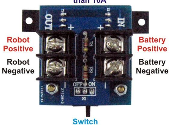
At the request of our customers we have now produced a high current, solid state switch for use with Wild Thumper products. Although designed specifically for the Wild Thumper chassis's this switch can be used with any robot that needs to switch high currents.
