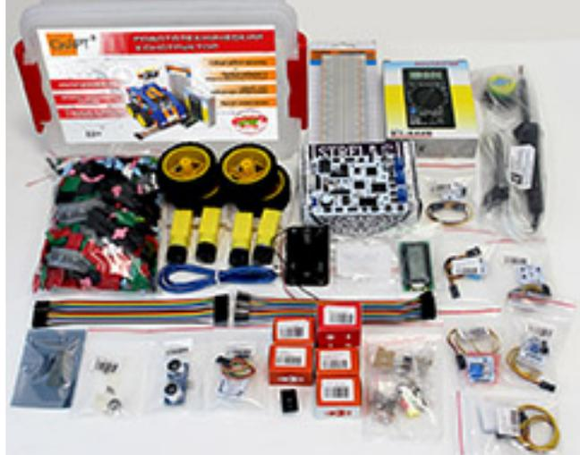
The image displays the contents of the SkART-3 kit. In addition to the sensors from the previous kits, it includes a 2-line LCD display, a breadboard, a multimeter, and various electronic components like resistors and integrated circuits. There are also more jumper wires and a small black module.                                                                                                                                                                        |
