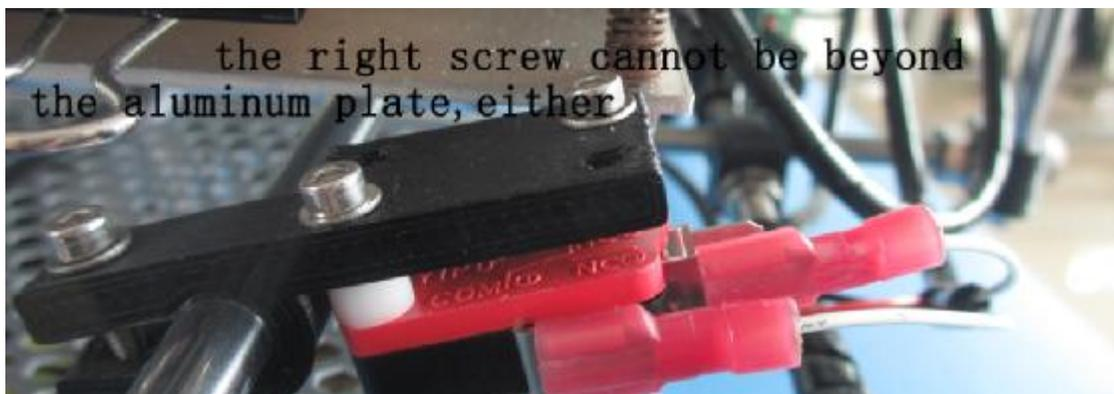
Z-axis end-stop position should be like the picture below,
