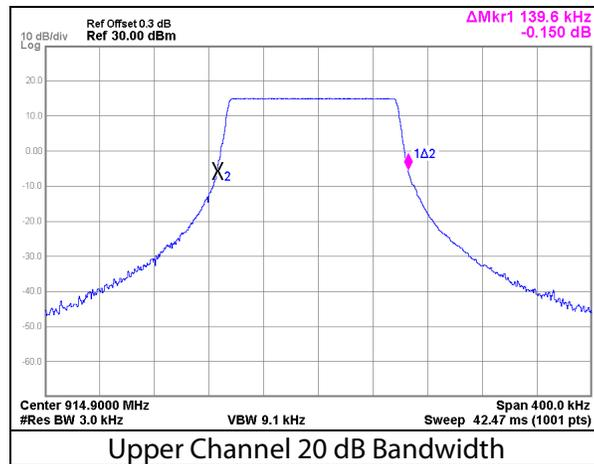
Figure 7: 20 dB BW Measurement
