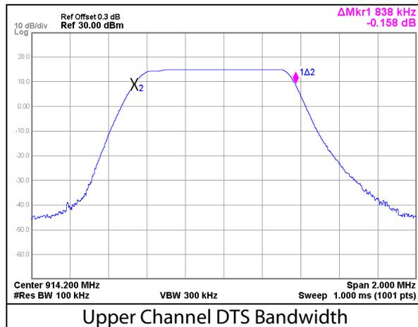
Figure 1: 6 dB BW Measurement
