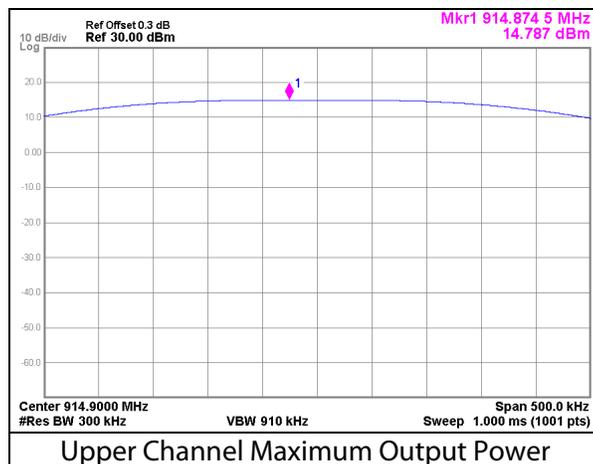
Figure 9: Peak Conducted Output Power Measurement
