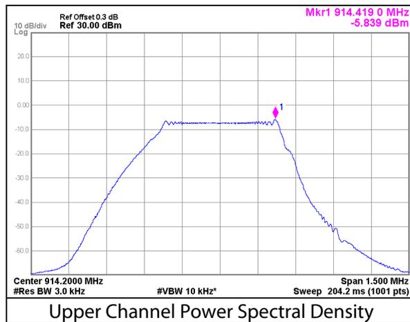
Figure 4: Power Spectral Density Measurement
