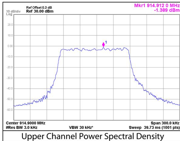
Figure 11: Power Spectral Density Measurement
