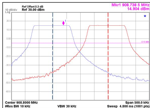
Figure 8: Measurement of Carrier Frequency Separation
