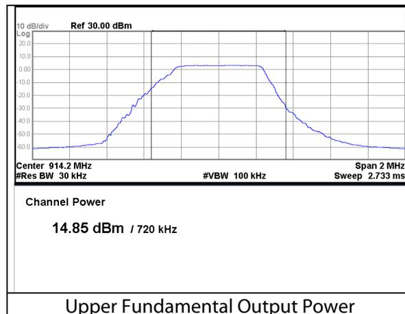
Figure 3: Fundamental Emission Output Power Measurement
