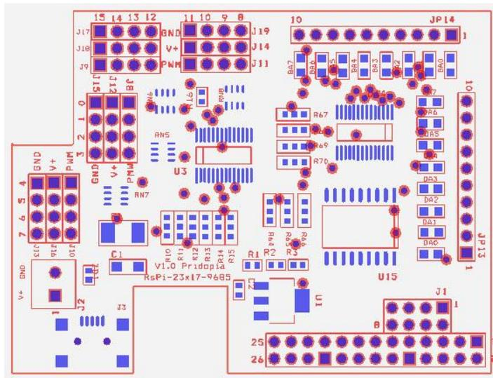
The PCA9685 is an I2C-bus controlled 16-channel LED controller optimized for LCD Red/Green/Blue/Amber (RGBA) color backlighting applications. Each LED output has its own 12-bit resolution (4096 steps) fixed frequency individual PWM controller that operates at a programmable frequency from a typical of 40 Hz to 1000 Hz with a duty cycle that is adjustable from 0 % to 100 % to allow the LED to be set to a specific brightness value.
