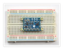
Place the 9DOF board right on top of the header so that the **short** pins are sticking thru the hole pads
