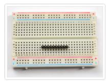
Start by breaking the header down so it is 10 pins long. Sometimes we toss in a longer strip, but its easy to break it down, just use pliers or diagonal cutters to snap it down to 10 pins.
