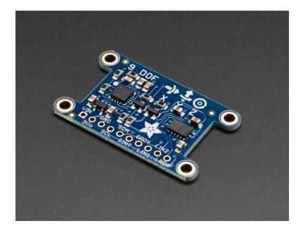
Adafruit's 9DOF (9 Degrees of Freedom) breakout board allows you to capture nine distinct types of motion or orientation related data: 3 degrees each of acceleration, magnetic orientation, and angular velocity.
