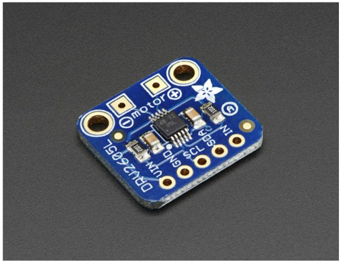
The DRV2605 from TI is a fancy little motor driver. Rather than controlling a stepper motor or DC motor, its designed specifically for controlling **haptic** motors - buzzers and vibration motors. Normally one would just turn those kinds of motors on and off, but this driver has the ability to have various *effects* when driving a vibe motor. For example, ramping the vibration level up and down, 'click' effects, different buzzer levels, or even having the vibration follow a musical/audio input.
