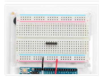
Prepare the header strip: Cut the strip to length if necessary. It will be easier to solder if you insert it into a breadboard - **long pins down**
