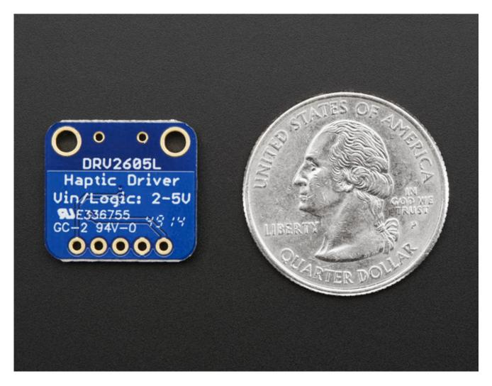
According to the product page, it can be used with both LRA (Linear Resonance Actuator) and ERM (Eccentric Rotating Mass) type motors but we have only used it with our little vibration pancake ERM. (http://adafru.it/dDc)
