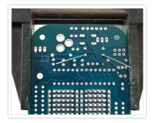
Now we will solder in the first part. Heat up your soldering iron (about 700 degrees F is common but you may need to adjust it higher for lead-free).
