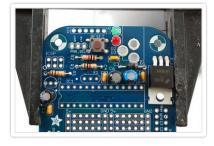
Now we will solder in the indicator LEDs. These LEDs are the Menta's way of telling you what's going on. LEDs are Light Emitting Diodes - which means that like the 1N4001 they have a polarity and won't work if placed backwards. Like capacitors, the also have a longer wire that indicates the **positive** lead. Place this wire in the hole marked with a +.
