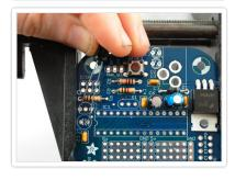
Next we will place the polarized electrolytic capacitors. These are the beefy versions of the ceramic capacitors we already placed. Ceramics are good for high frequency noise, and the electrolytics are good for low frequency noise, that's why we team them up together to cover all frequencies.
