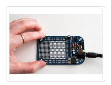
Now we can do a test, find a DC power adapter, 7VDC or higher, with a 2.1mm jack and center-polarity (these are nearly standard) and plug it in. With the jumper in place, you should see the Green LED light up. If not, something is wrong either the LED is in backwards or your power supply isn't working. Go back and check your work until you can figure out what happened.
