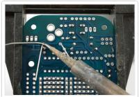
Now we will place our first non-symmetric component, a diode! The diode only conducts current in one direction. We use this diode for protecting the Menta - since it can only work in one direction it makes sure we don't connect negative voltages into the DC plug that could damage or destroy the electronics. This particular diode is a **1N4001** model, which is extremely common power diode that can handle over an Amp of current.
