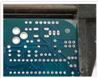
Using your diagonal cutters, cut off the long leads just above the solder joint.
