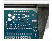
Flip over the PCB and solder the 2 resistors.
