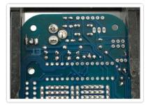
Next up is the 16.00 MHz crystal **X1**. This crystal is what lets the Menta chip run at a brisk 16 million clocks per second. This oscillator comes in a orange shape with three pins. Luckily, it's symmetric so just place it any way you like.
