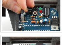
working, we can continue. Next up we will solder in the 3.3V regulator. This will let us power the many 3.3V sensors and accessories out there, a nice little extra! The chip we'll be using is the MCP1700-330 - you should be able to see this marking on the face of the little chip. This regulator can supply up to 250mA, which is plenty for nearly any device you'll be using. Place the chip so that the flat face matches the flattened image silkscreened on the PCB.
