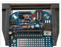
Next, we will be placing the 28-pin socket next to it. This socket is a mechanical 'holder' - it holds the ATmega328 chip that drives the Menta. We socket it for a few reasons - one to protect the chip, to make it easier to replace in case of damage, and so that you don't have to worry about accidentally soldering it in backwards. If you mess up on the socket, it's a lot easier to fix than if you do the same with the chip.
