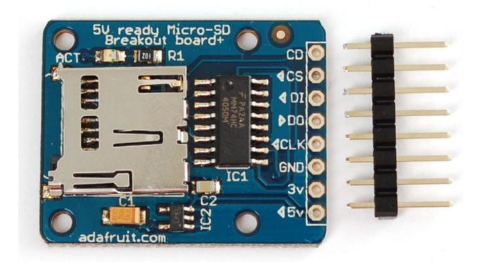
If you have a project with any audio, video, graphics, data logging, etc in it, you'll find that having a removable storage option is essential. Most microcontrollers have extremely limited built-in storage. For example, even the Arduino Mega chip (the Atmega2560) has a mere 4Kbytes of EEPROM storage. There's more flash (256K) but you can't write to it as easily and you have to be careful if you want to store information in flash that you don't overwrite the program itself!
