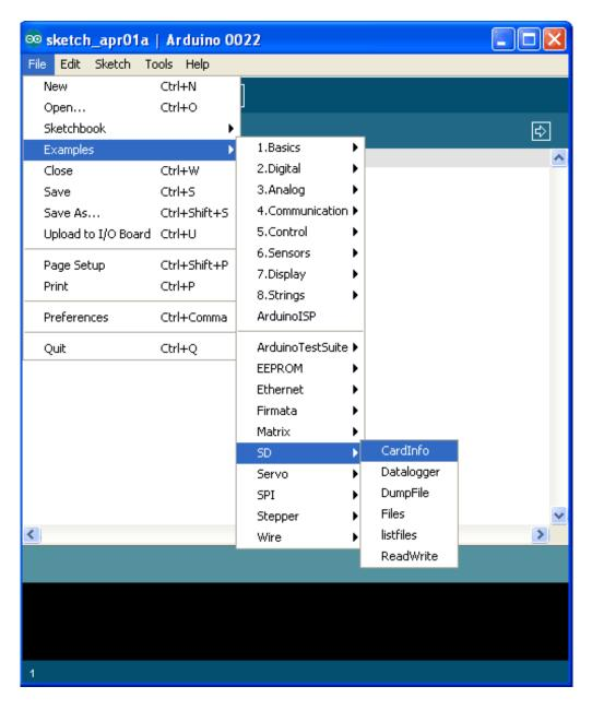
This sketch will not write any data to the card, just tell you if it managed to recognize it, and some information about it. This can be **very** useful when trying to figure out whether an SD
