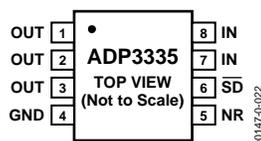
Figure 3. 8-Lead MSOP
