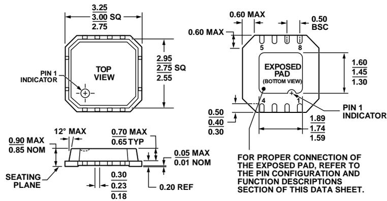
Figure 26. 8-Lead Lead Frame Chip Scale Package [LFCSP\_VD]
