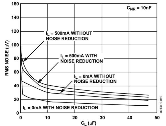
Figure 21. RMS Noise versus  $C_L$  (10 Hz to 100 kHz)
