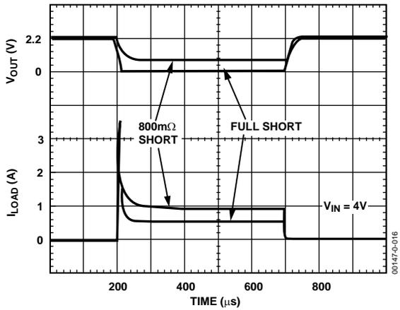
Figure 18. Short-Circuit Current
