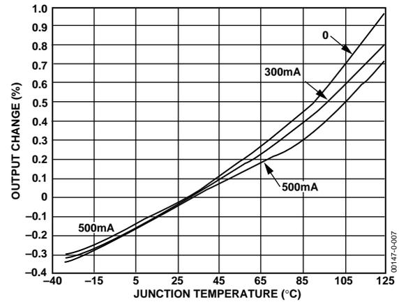
Figure 9. Output Voltage Variation vs. Junction Temperature
