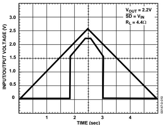
Figure 12. Power-Up/Power-Down
