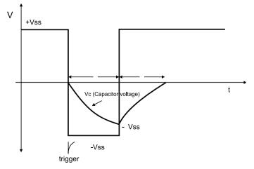
Figure 2.6: Monostable Multivibrator and its outputs
