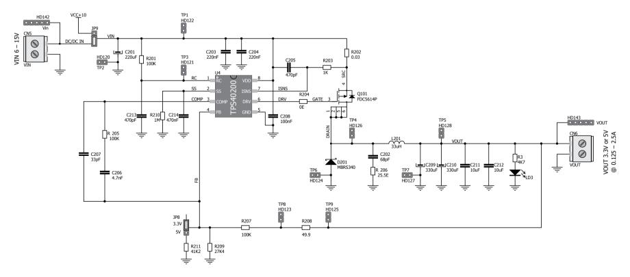
Figure 12.1: Schematic of the on-board EVM
