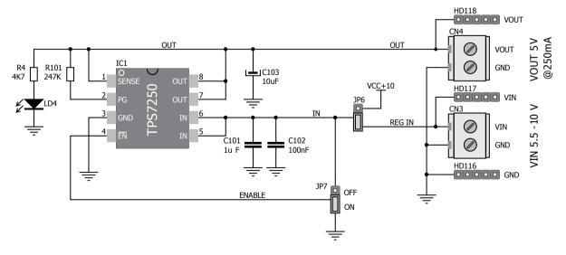
Figure 11.1: Schematic diagram of on-board evaluation module
