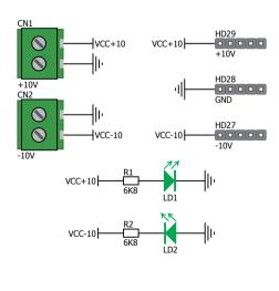
Figure D.18: Main power supply
