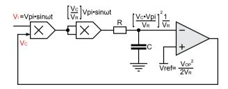
Figure 8.1: Automatic Gain Control (AGC)/Automatic Volume Control (AVC)
