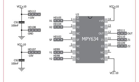
Figure D.9: Connections for analog multiplier MPY634 - SET III
