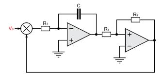
Figure 6.3: Voltage-Controlled Oscillator (VCO)
