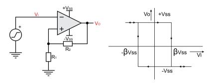
Figure 2.1: Inverting Schmitt-Trigger and its Hysteresis Characteristic
