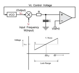
Figure 7.1: Phase Locked Loop (PLL) and its characteristics
