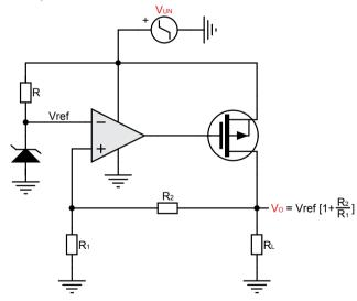
Figure 10.1: Low Dropout Regulator (LDO)
