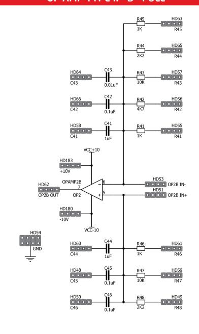
Figure D.4: OP-Amp 2B can be used in both inverting and non-inverting configuration
