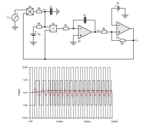
Figure 7.2: Sample output waveform for the Phase Locked Loop (PLL) Experiment
