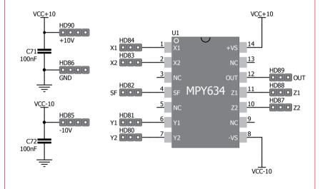
Figure D.7: Connections for analog multiplier MPY634 - SET I
