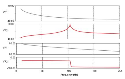
Figure 3.3: Frequency Response of integrator and differentiator
