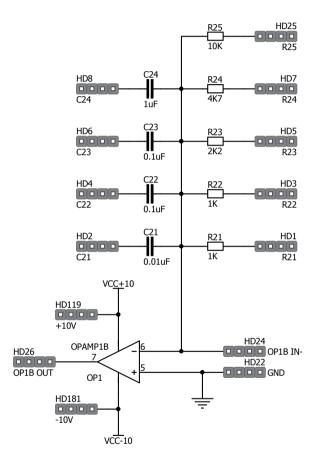
Figure D.2: OP-Amp 1B connected in inverting configuration
