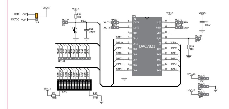
Figure D.10: connections for analog-to-digital converter DAC7821 - DAC I
