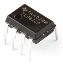
Figure A.1: TL082 - IFET-Input Operational Amplifier
