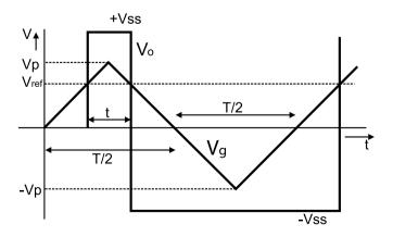
Figure 9.1: DC-DC Converter and PWM waveform
