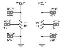
Figure D.17: Trimmer-potentiometers
