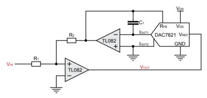
Figure 13.1: Circuit for Digital Controlled Gain Stage Amplifier
