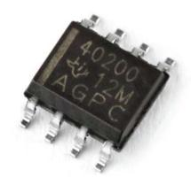
Figure A.4: TPS40200 - DC/DC Controller
