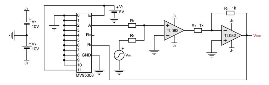
Figure 13.2: Equivalent Circuit for simulation
