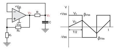
Figure 2.4: Astable Multivibrator and its characteristics
