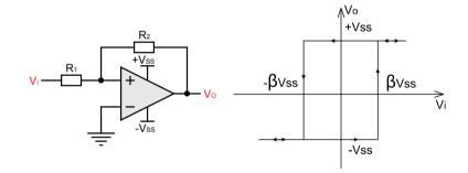
Figure 2.3: Non-inverting Schmitt Trigger and its Hysteresis Curve
