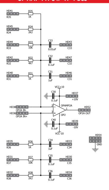
Figure D.3: OP-Amp 2A can be used in both inverting and non-inverting configuration
