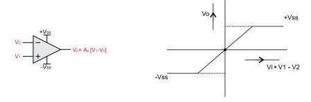
Figure 1.1: An ideal Dual-Input, Single-Output OP-Amp and its I-O characteristic
