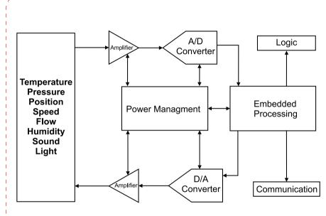
Figure: Signal Chain in an Electronic System
