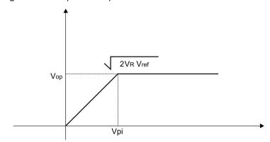
Figure 8.2: Input-Output Characteristics of AGC/AVC
