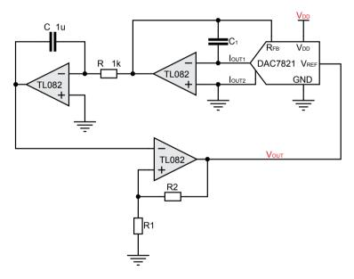
Figure 14.1: Circuit for Digital Controlled Oscillator
