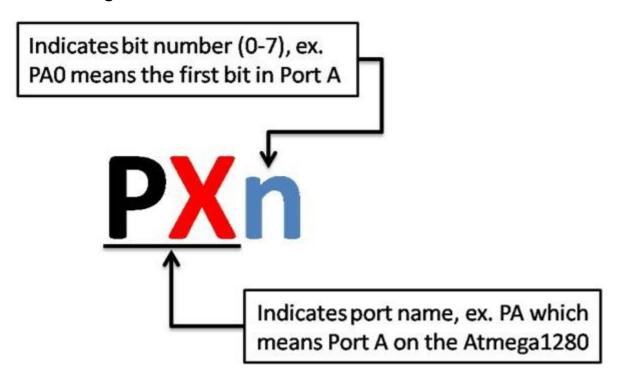
**Note:** Port names and numbering in the Seeeduino Mega matches the port naming and numbering convension of Atmega1280's datasheet.
