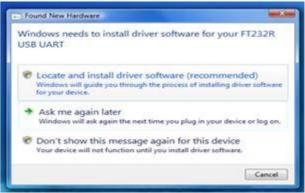
\*After the driver installation, go to My Computer > Properties > Device Manager then look for Ports (COM and LPT) > USB Serial Port (COMn) the n may vary from one PC to another, in this case we have 4. Take note of this since it will be used in the Arduino IDE configuration.
