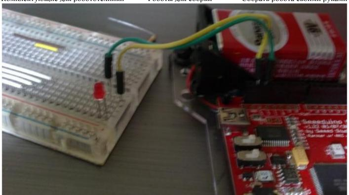
Green is Pin13 while Yellow in Ground, in this set up I used a 3.5mm LED the maximum current that should be forced to it must be below 10mA. However to have a brighter blink I omitted the series resistor - thus in order to dim the output just add a resistor in series of the LED. Also take note that an LED's legs can't be and shouldn't be interchanged. See <a href="http://en.wikipedia.org/wiki/Light-emitting\_diode">http://en.wikipedia.org/wiki/Light-emitting\_diode</a> for more details.
