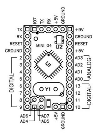
*Pin out of the Arduino Mini 04.* (Note that the ground pin on the left has moved down one pin.)
