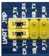
Figure 2: Starting up serial debugging function
