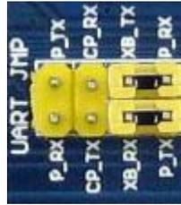
Figure 14: Setting jumpers on ARPI600
