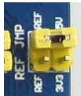
Figure 18: Setting AD reference voltage
