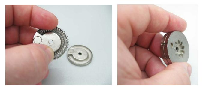
Now fit the clutch onto the servo and rotate the servo fully clockwise. This will be the servos position when the gripper is fully closed. This step is very important to ensure the servo and mechanism is correctly aligned.
