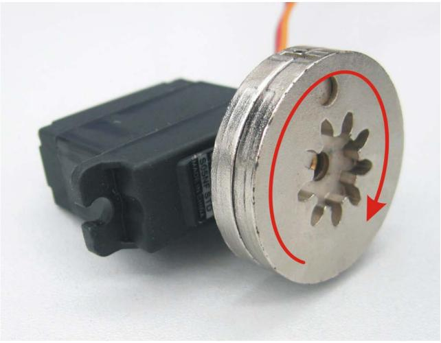
Slide the servo and clutch assembly into the gripper and mount with the screws provided. Do not over-tighten the servo mounting screws.
