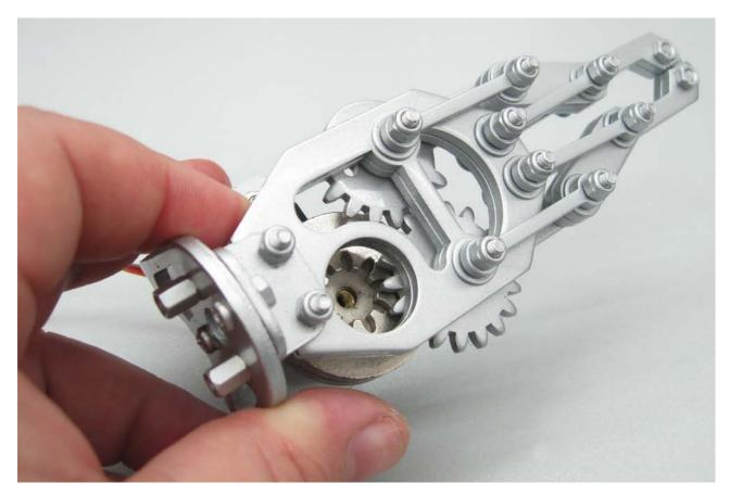
If necessary you may need to force the clutch to slip slightly to get the teeth of the gears to align. Install the clutch pinion gear, brass sleeve and mount them with the screw provided.
