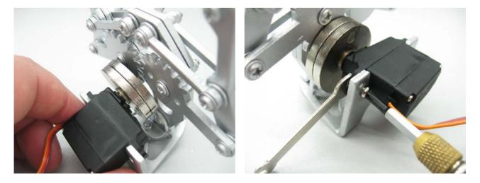
Now move the gripper to the fully closed position. As the servo was also moved to the fully closed position in the previous step they should now be aligned.
