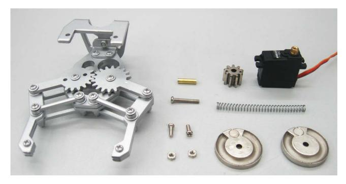
Start by installing the spring in the clutch. Hold the spring in place with one hand while you place the other half on top. When the two halves are joined the magnets will hold the assembly together. The main purpose of the magnets is to lock the clutch when it is not under excessive load.
