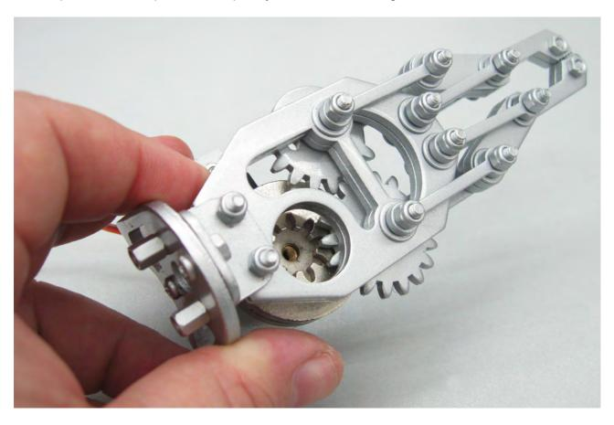
If necessary you may need to force the clutch to slip slightly to get the teeth of the gears to align. Install the clutch pinion gear, brass sleeve and mount them with the screw provided.
