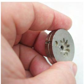
Now fit the clutch onto the servo and rotate the servo fully clockwise. This will be the servos position when the gripper is fully closed. This step is very important to ensure the servo and mechanism is correctly aligned.
