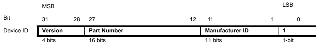
Figure 27-1. The Format of the Device Identification Register
