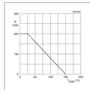
Fig.4 Maximum permissible continuous forward current as a function of ambient temperature.
