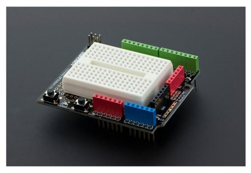
This is a design for an open-source prototyping shield for Arduino NG/Diecimila. It has tons of cool features, to make prototyping on your Arduino easy. Shipped with fully assembled.
