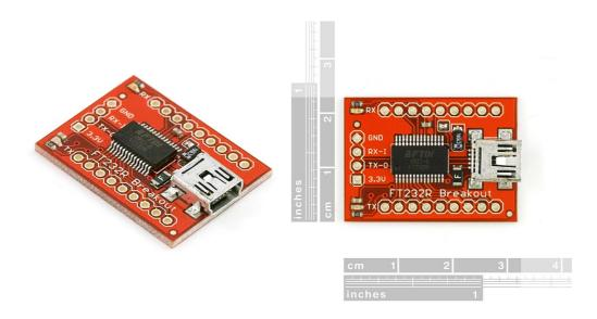
**Description:** Basic breakout board for FTDI's popular USB to UART IC. Now with internal oscillator and EEPROM, the FT232RL is an impressive IC!
