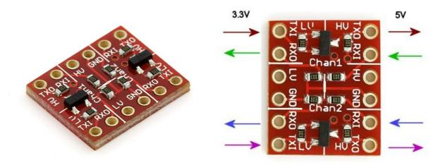
**Description:** If you've ever tried to connect a 3.3V device to a 5V system, you know what a challenge it can be. The SparkFun logic level converter is a small device that safely steps down 5V signals to 3.3V and steps up 3.3V to 5V. This level converter also works with 2.8V and 1.8V devices. Each level converter has the capability of converting 4 pins on the high side to 4 pins on the low side. Two inputs and two outputs are provided for each side.
