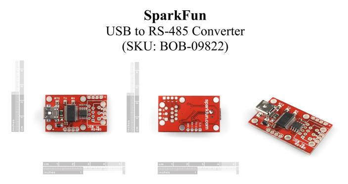
**Description:** This is the newest revision and fixes issues with the last board. This breakout board pairs an SP3485 RS-485 transceiver with an FT232RL USB UART IC to convert a USB stream to RS-485. The SP3485 is a half-duplex transceiver, so it can only communicate one way at a time, but it can reach transmission speeds of up to 10Mbps.
