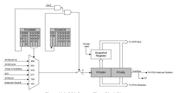
Figure 19.2. PCA Counter/Timer Block Diagram
