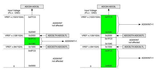
Figure 5.16. ADC Window Compare Example: Left-Justified Single-Ended Data
