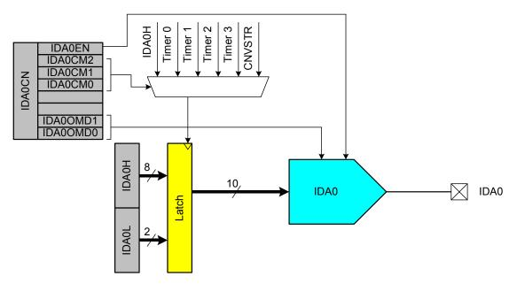
Figure 1.12. IDA0 Functional Block Diagram
