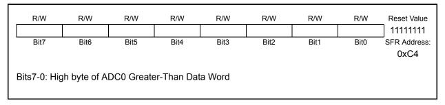
Figure 5.11. ADC0GTH: ADC0 Greater-Than Data High Byte Register
