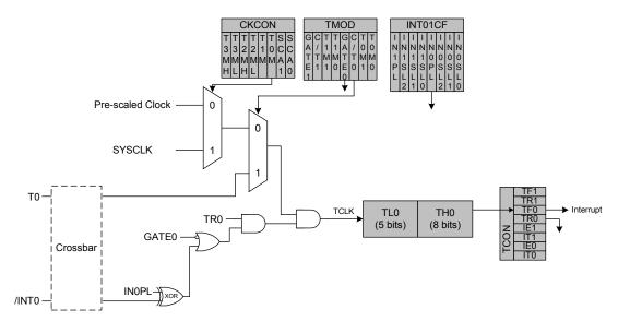
Figure 18.1. T0 Mode 0 Block Diagram
