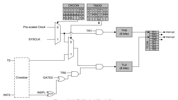
Figure 18.3. T0 Mode 3 Block Diagram
