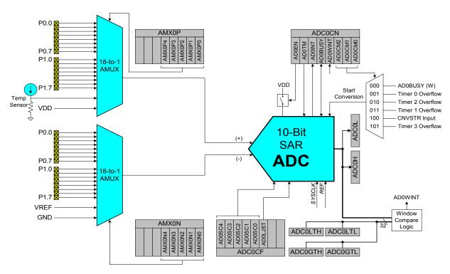
Figure 5.1. ADC0 Functional Block Diagram
