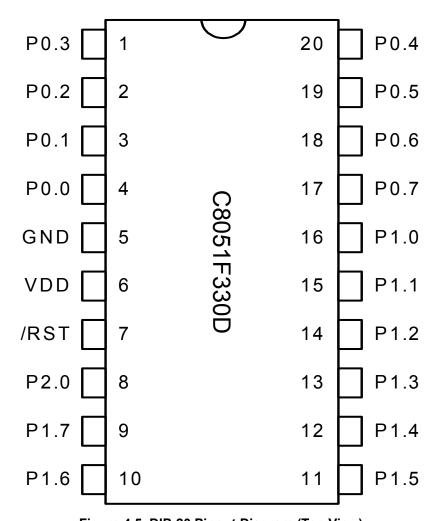
Figure 4.5. DIP-20 Pinout Diagram (Top View)
