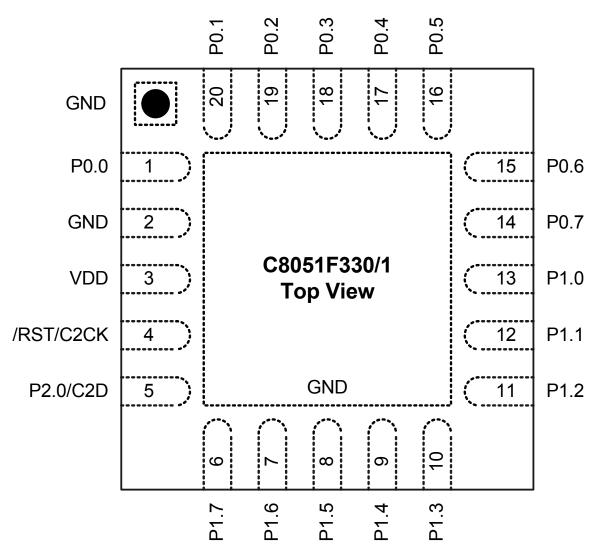
Figure 4.1. MLP-20 Pinout Diagram (Top View)
