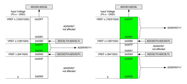
Figure 5.15. ADC Window Compare Example: Right-Justified Single-Ended Data
