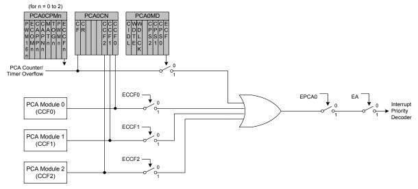
Figure 19.3. PCA Interrupt Block Diagram
