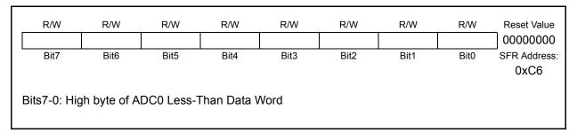
Figure 5.13. ADC0LTH: ADC0 Less-Than Data High Byte Register
