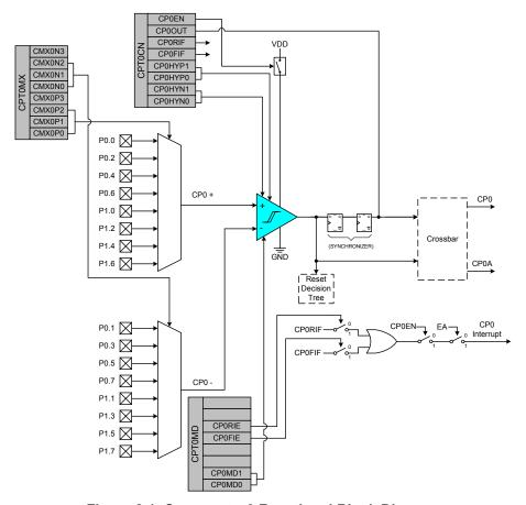
Figure 8.1. Comparator0 Functional Block Diagram
