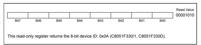
Figure 20.2. DEVICEID: C2 Device ID Register
