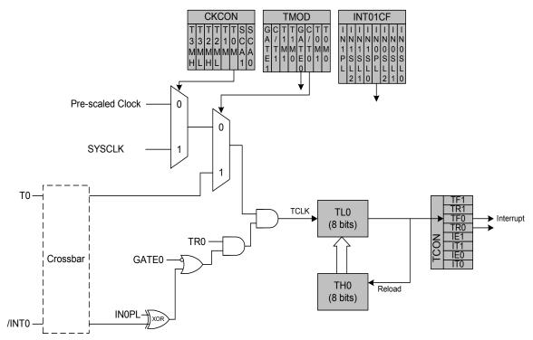
Figure 18.2. T0 Mode 2 Block Diagram
