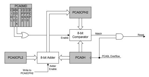
Figure 19.10. PCA Module 2 with Watchdog Timer Enabled
