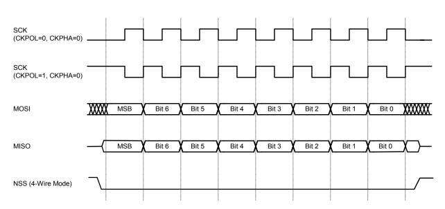
Figure 17.6. Slave Mode Data/Clock Timing (CKPHA = 0)
