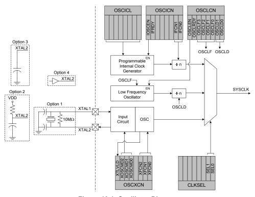
Figure 13.1. Oscillator Diagram
