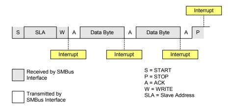
Figure 15.10. Typical Slave Receiver Sequence
