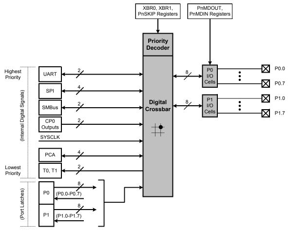
Figure 14.1. Port I/O Functional Block Diagram
