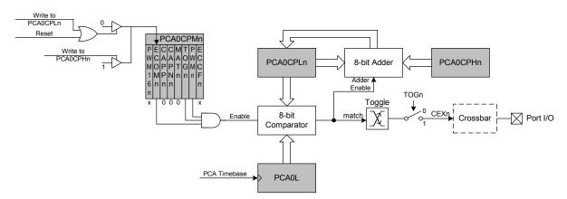
Figure 19.7. PCA Frequency Output Mode
