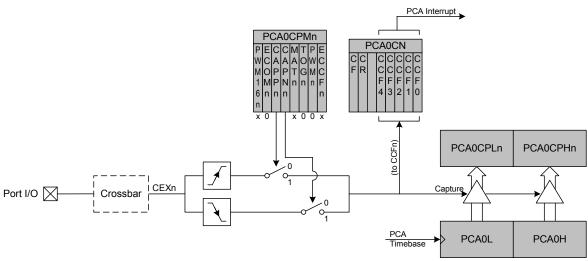
Figure 19.4. PCA Capture Mode Diagram
