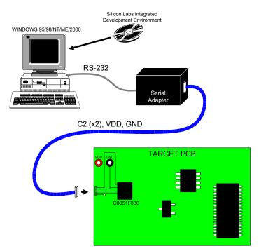
Figure 1.6. Development/In-System Debug Diagram
