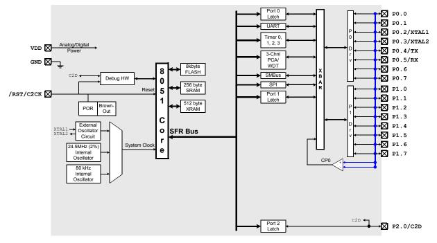
Figure 1.2. C8051F331 Block Diagram
