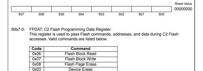
Figure 20.5. FPDAT: C2 Flash Programming Data Register
