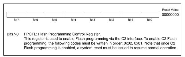
Figure 20.4. FPCTL: C2 Flash Programming Control Register
