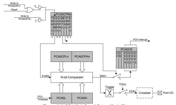
Figure 19.6. PCA High-Speed Output Mode Diagram
