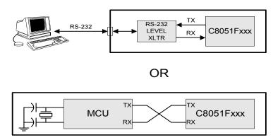
Figure 16.3. UART Interconnect Diagram
