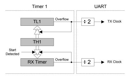
Figure 16.2. UART0 Baud Rate Logic
