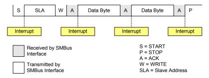
Figure 15.8. Typical Master Transmitter Sequence
