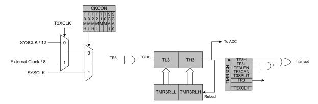
Figure 18.18. Timer 3 16-Bit Mode Block Diagram
