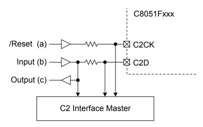
Figure 20.6. Typical C2 Pin Sharing
