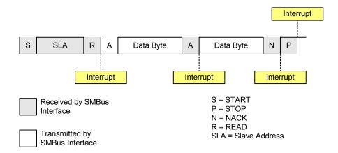
Figure 15.11. Typical Slave Transmitter Sequence
