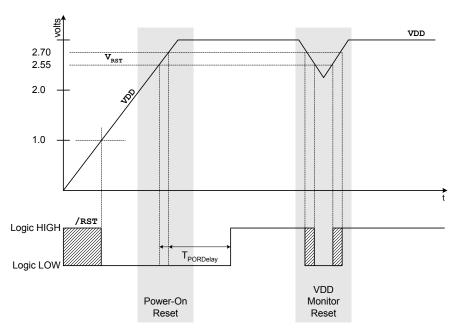
Figure 10.2. Power-On and  $V_{DD}$  Monitor Reset Timing
