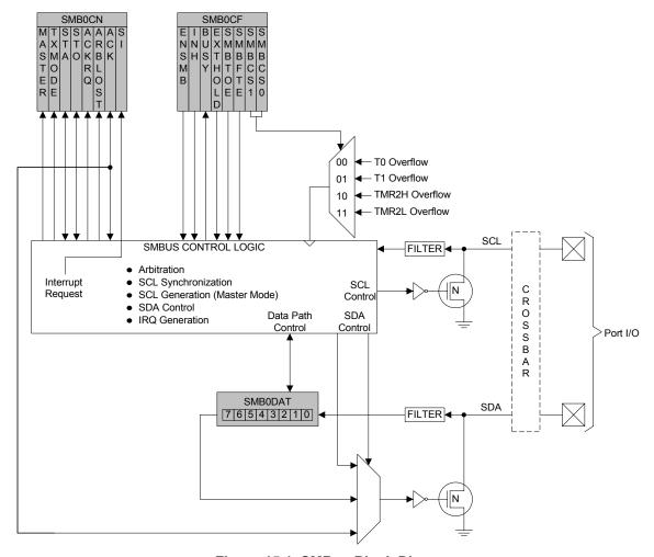
Figure 15.1. SMBus Block Diagram
