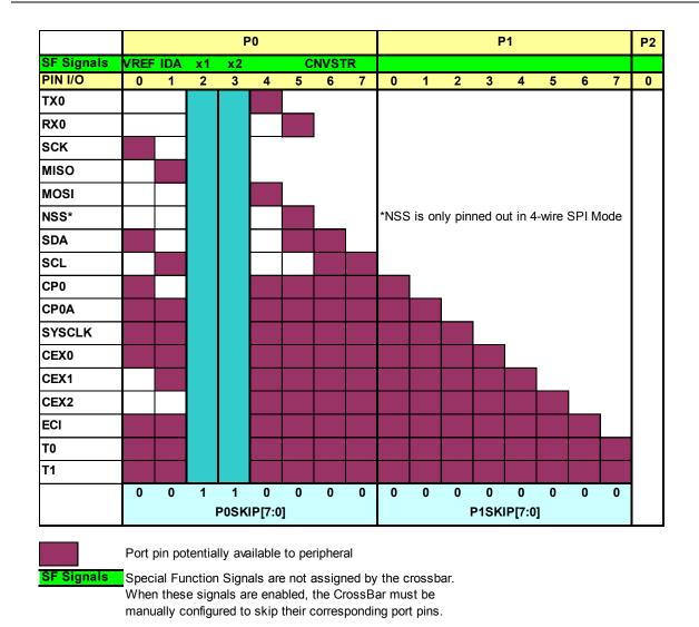
Figure 14.4. Crossbar Priority Decoder with Crystal Pins Skipped
