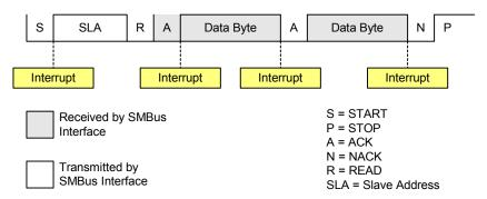
Figure 15.9. Typical Master Receiver Sequence
