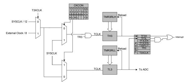
Figure 18.19. Timer 3 8-Bit Mode Block Diagram
