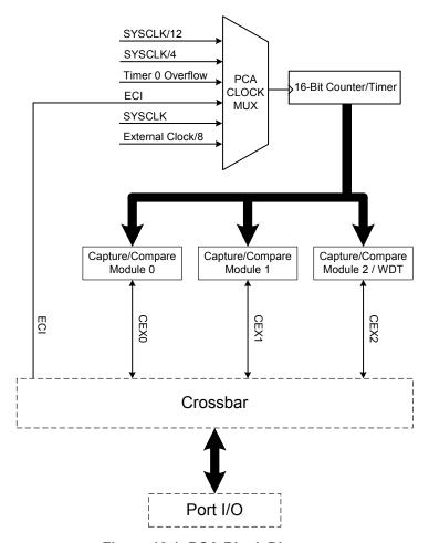
Figure 19.1. PCA Block Diagram
