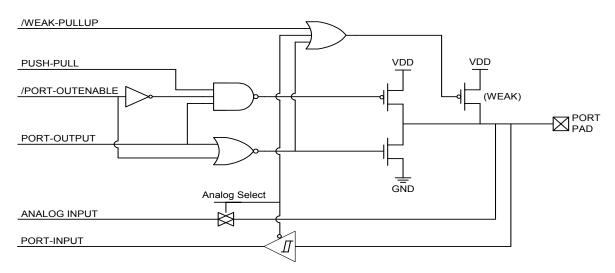
Figure 14.2. Port I/O Cell Block Diagram
