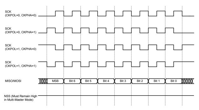
Figure 17.5. Master Mode Data/Clock Timing
