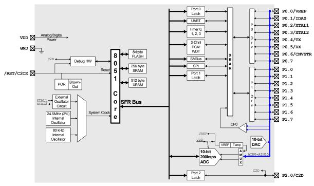
Figure 1.1. C8051F330 and C8051F330D Block Diagram
