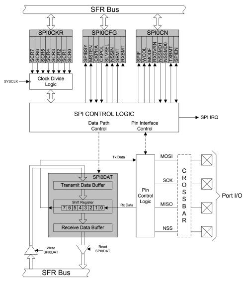
Figure 17.1. SPI Block Diagram
