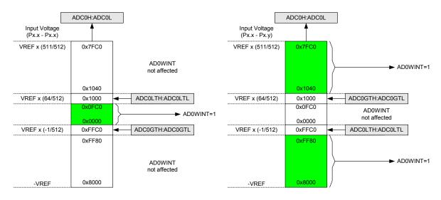
Figure 5.18. ADC Window Compare Example: Left-Justified Differential Data
