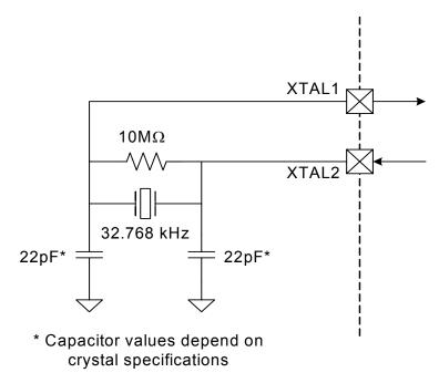
Figure 13.6. External 32.768 kHz Quartz Crystal Oscillator Connection Diagram
