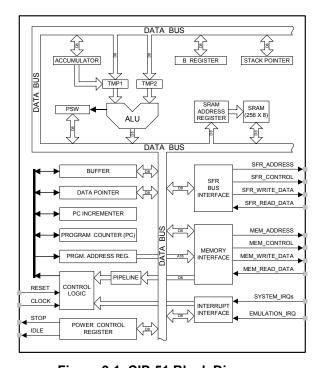
Figure 9.1. CIP-51 Block Diagram
