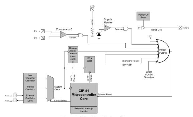
Figure 1.4. On-Chip Clock and Reset
