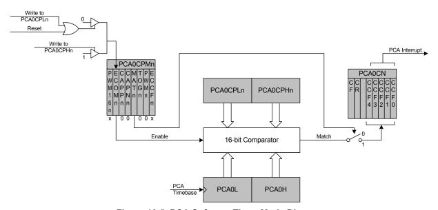
Figure 19.5. PCA Software Timer Mode Diagram
