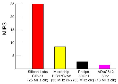
Figure 1.3. Comparison of Peak MCU Execution Speeds
