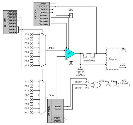
Figure 1.11. Comparator Block Diagram
