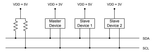
Figure 15.2. Typical SMBus Configuration
