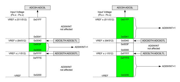
Figure 5.17. ADC Window Compare Example: Right-Justified Differential Data
