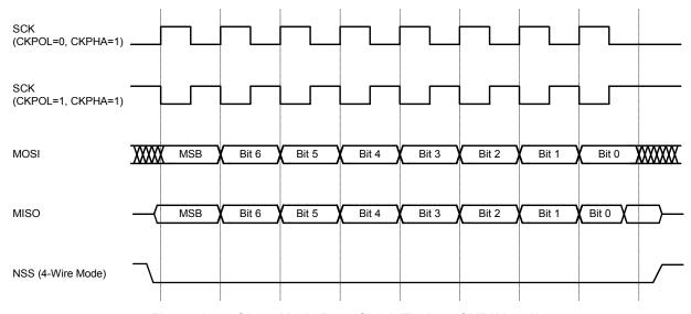
Figure 17.7. Slave Mode Data/Clock Timing (CKPHA = 1)
