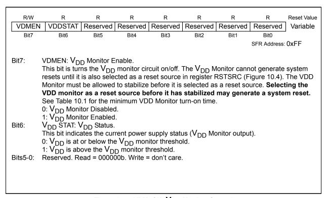
Figure 10.3. VDM0CN: V<sub>DD</sub> Monitor Control
