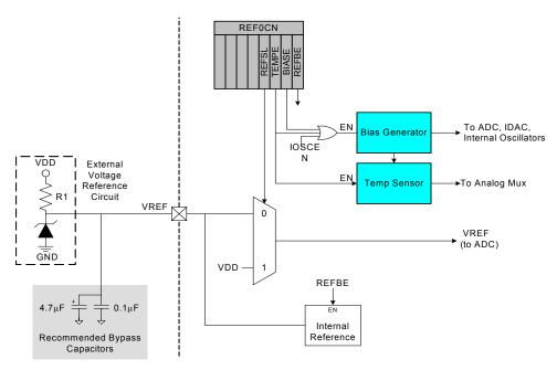
Figure 7.1. Voltage Reference Functional Block Diagram
