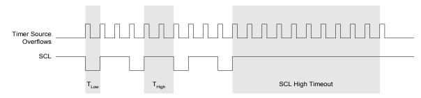
Figure 15.4. Typical SMBus SCL Generation
