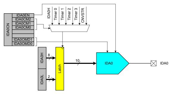
Figure 6.1. IDA0 Functional Block Diagram
