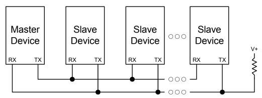
Figure 16.6. UART Multi-Processor Mode Interconnect Diagram
