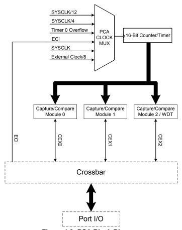
Figure 1.9. PCA Block Diagram
