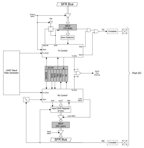
Figure 16.1. UART0 Block Diagram
