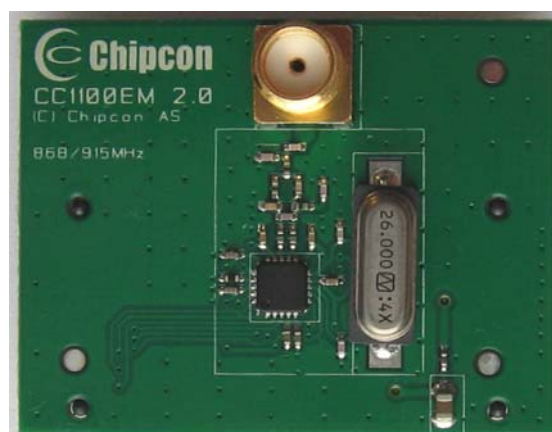
Figure 6: CC1100EM reference design, 868/915 MHz
