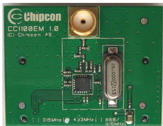
Figure 5: CC1100EM reference design, 433 MHz. Same PCB is used for 315 MHz
