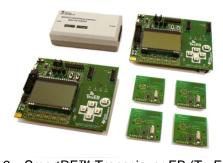
2 x SmartRF™ Transciever EB (TrxEB) 2 x CC110LEM 868/915 MHz 1 x CC113LEM 868/915 MHz 1 x CC115LEM 868/915 MHz 1 x MSP430 Debug Probe (FET) 2 x Micro USB Cables 1 x Standard USB Cable 1 x 14-pin Flat Cable 4 x 1.5 Volt AA Batteries Documentation
