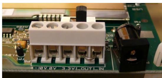
The second method applies DC power using the DC input jack (right in picture, centre is +, sleeve is ground), or by connecting a 4-10V voltage source between the 4-10V and 0V terminals of the power connector (left in picture). It is also possible to connect a 3.3V voltage source between the 3.3V and 0V terminals. The on-board voltage regulators will be bypassed in this case.
