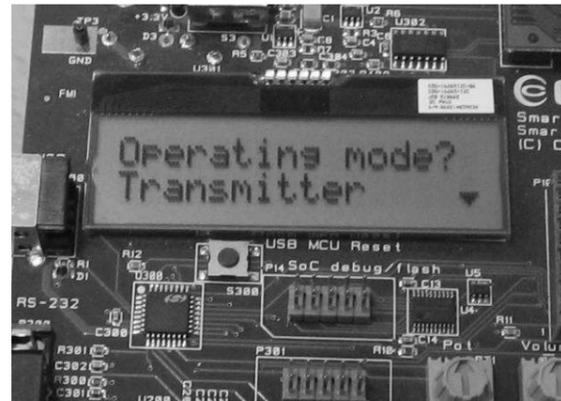
Select Transmitter on the other EB by moving the joystick upward. Confirm by pressing button S1.
