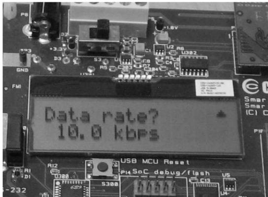
Select which data rate to use (10 kbps, 250 kbps or 500 kbps) by moving the joystick. Confirm your choice by pushing button S1.
