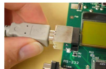
The EB can also be powered from the USB bus. Make sure that the SmartRF™ Studio software is installed before connecting the EB to the PC; otherwise you may experience problems in installing it later due to driver issues.
