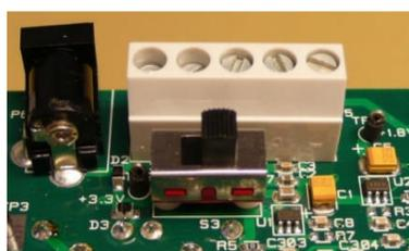
If a 3.3V source is used as described in 4b above, the switch should be set to the leftmost position. For all other cases, the switch should be set to the rightmost position. This switch can be used to turn off the EB by switching it to the opposite position of that used to turn it on.
