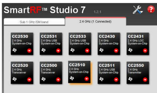
After installing the tool, connect the EB to the PC using the USB cable and start SmartRF Studio. Select the "2.4 GHz" tab and double click the CC2510 device icon.
