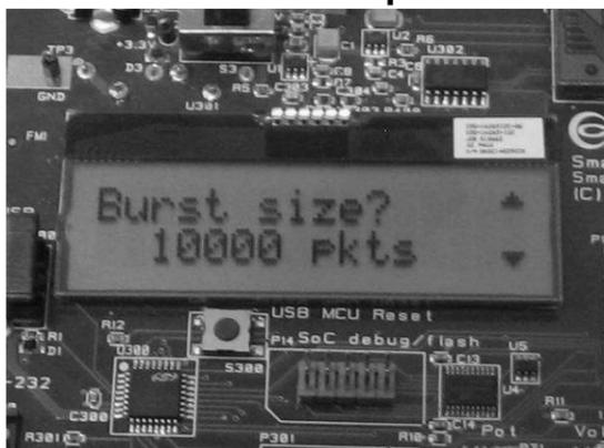
On the transmitter EB, select the number of packets to send. More packets take longer, but give a better statistical result. Confirm by pressing button S1.
