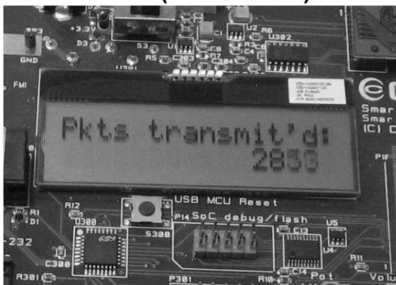
Press S1 button again to start transmitting the packet burst. The transmitter will show a running counter that shows the number of packets sent.
