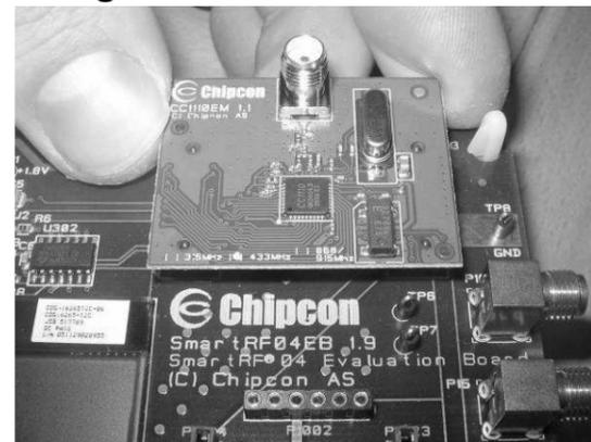
Insert a CC2510EM into both SmartRF04EBs. The connectors will only fit in one position, so that the EM cannot be inserted the wrong way. Do not force the EM. Remember to mount the antenna as well.
