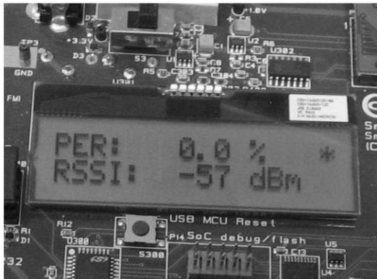
When the PER test is completed, the result will be displayed on the receiver until a new test is started. A new test can be started from the transmitter.
