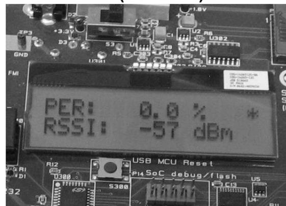
The receiver will show the total accumulated packet error rate (PER) together with the average signal strength (RSSI) of the previous 32 received packets. A symbol in the upper right corner will blink for every 32nd incoming packet to indicate whether the link is maintained.
