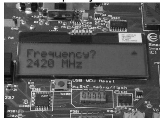
Select the frequency that you want to use (2420 MHz, 2440 MHz, 2460 MHz or 2480 MHz). Move the joystick up or down to display the choices and push button S1 in the lower right corner of the board to select the displayed frequency.
