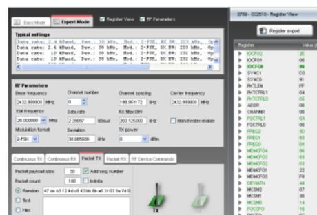
You can now configure the radio, run tests, export register settings and run link tests with another CC2510 on a SmartRF04EB connected to the PC.
